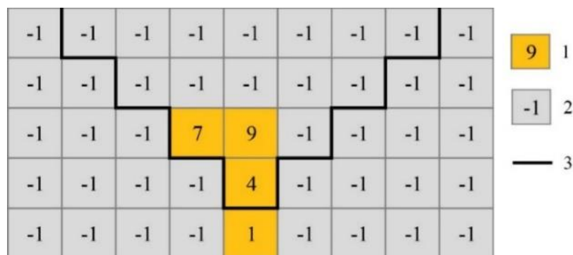
Figure 1. Simplified Visualization of the Lerchs-Grossmann algorithm. Legend: 1 – mineralized blocks with estimated value, 2 – waste blocks with estimated value, 3 – open pit boundary.
